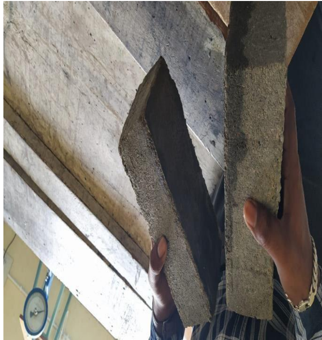
Fig 8.6 Soundness Test on Bricks
