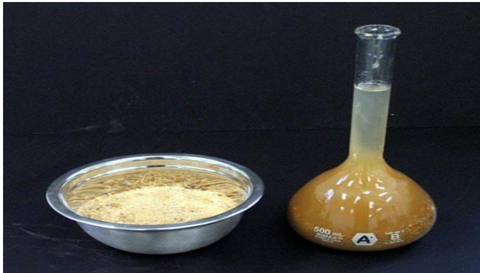
Fig 7.5 Specific gravity Using Pycnometer
