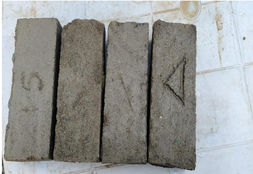
Fig 8.1 Water Absorption of Bricks
