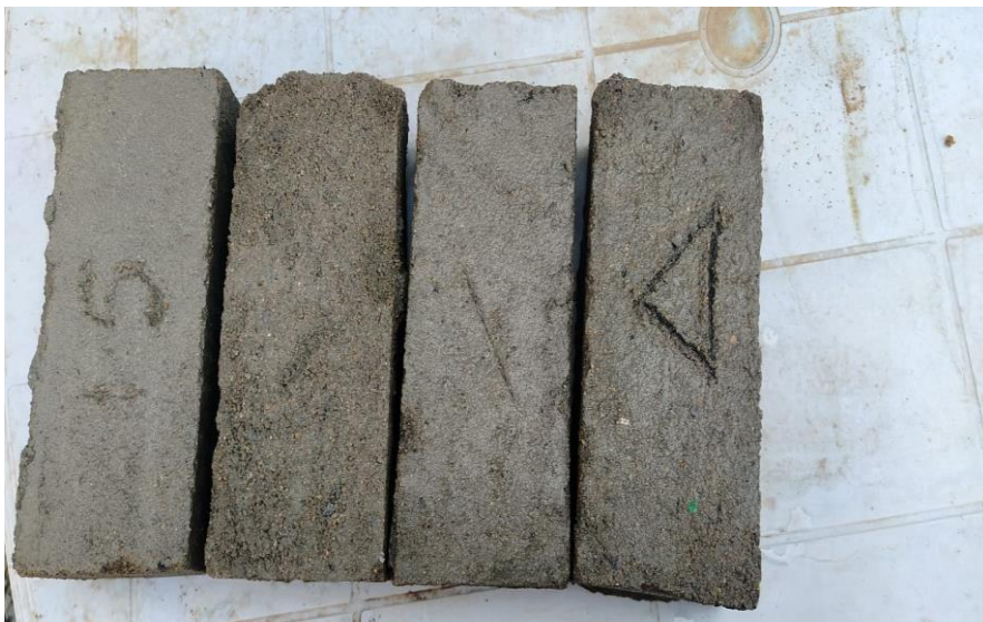
Fig 8.4 Efflorescence test on Bricks
